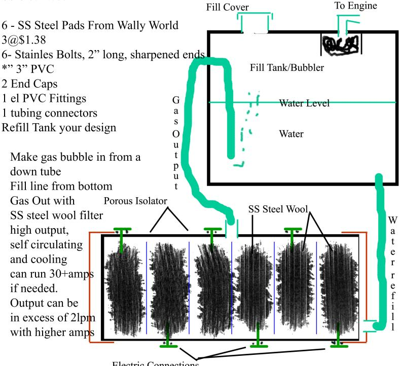
**Electric Connections** Glue and Seal end cap 1 (on Left) Modify 3" tube with straight fitting Drill and taps holes at 5/8, +21/2, +21/2 from left of tube on one side drill and tap holes at  $1 \frac{7}{8}$ ,  $+2 \frac{1}{2}$ ,  $+2 \frac{1}{2}$  from left side opposite side, or at 90 degrees from first side. Insert screws with wire connections, and seals and check for shorts.
